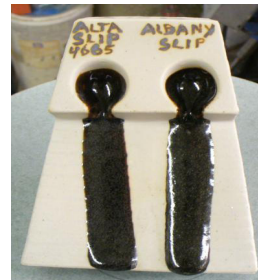
Cone 10R melt flow test showing Alberta Slip beside Albany Slip. Alberta Slip duplicates the chemistry and firing characteristics of Albany Slip.
