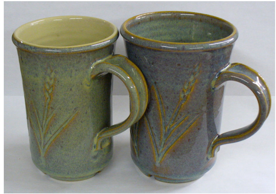
Adding 20% Ferro Frit 3134 to Alberta Slip produces a base that melts very well at cone 6. GA6-C (left) and GA6-E (right) simply add 4% rutile to get a stunning blue (E adds an additional 4% spodumene).
